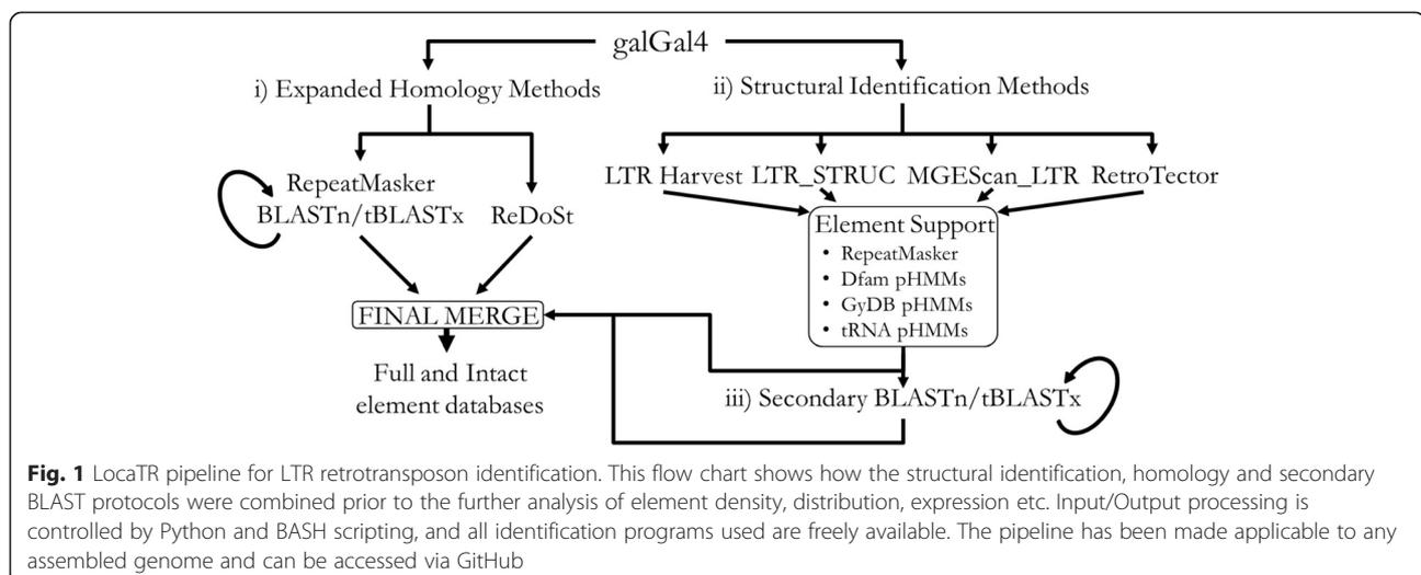
**Fig. 1** LocaTR pipeline for LTR retrotransposon identification. This flow chart shows how the structural identification, homology and secondary BLAST protocols were combined prior to the further analysis of element density, distribution, expression etc. Input/Output processing is controlled by Python and BASH scripting, and all identification programs used are freely available. The pipeline has been made applicable to any assembled genome and can be accessed via GitHub
