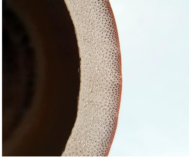
Figure 1 Cross section of bamboo culm showing a non-uniform distribution of fibres through the thickness.
