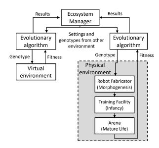
Figure 3: Diagram of the ARE system components: the virtual environment, the physical environment, and the Ecosystem Manager. Simulated and physical evolution are running concurrently, supervised and controlled by the Ecosystem Manager.
