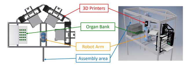
Figure 6: Concept layout for the final Robot Fabricator design to facilitate automated production of complete robots. The skeleton is printed on one or more printers, and assembled by the robot arm together with organs from the organ bank.
