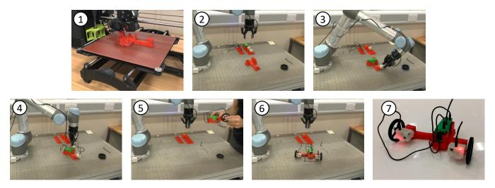
Figure 7: Robot production: (1) skeleton is 3D printed, (2), manual transfer to assembly area, (3) organs attached, (4) cables connected between organs, (5) manual wheel attachment, (6) robot is finished and (7) is tested. These images are from a video which is available online at www.york.ac.uk/robot-lab/are/alife2019/.
