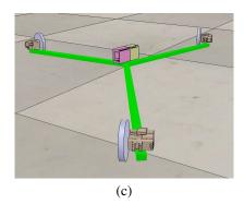
Figure 10: Examples of robots evolved without viability test: (a) robot with overlapping organs, (b) robot with high number of organs and (c) robot bigger than build volume.
