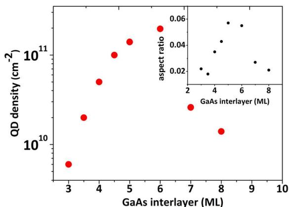
FIG. 2. Variation of QD density versus GaAs interlayer thickness. The inset shows the QD aspect ratio as function of the interlayer.  $\text{In}_{0.5}\text{Ga}_{0.5}\text{Sb}$  coverage is kept fixed to 0.42 ML.
