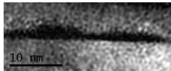
FIG. 6. Amplitude of the Fourier-filtered (200)-reflection of a [010]-zone axis HRTEM image of single 0.42 ML  $\text{In}_{0.5}\text{Ga}_{0.5}\text{Sb}$  QDs on 5 ML GaAs/GaP with 15 s GRI and 6 nm GaP capping layer. They were grown without any Sb-Flush. The dark region represents a material contrast whereby the QDs can be easily recognizable.
