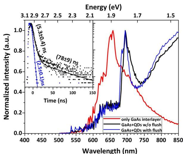
FIG. 7. PL spectra at 10 K of  $\text{In}_{0.5}\text{Ga}_{0.5}\text{Sb}$  QDs on 5 ML GaAs/GaP: (blue) with Sb-flush; (black) without Sb-flush; (red) no QDs, only 5 ML GaAs/GaP; normalized to 1.0. Inset: Time-resolved PL transients (at 4 K) recorded at 695 nm emission wavelengths for  $\text{In}_{0.5}\text{Ga}_{0.5}\text{Sb}$  QDs grown with (blue) and without (black) Sb-flush. Solid lines show mono- or bi-exponential fits to the data.
