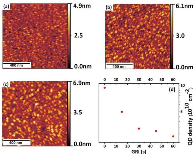
FIG. 4. (a)–(c) AFM measurements of 0.9 ML  $\text{In}_{0.5}\text{Ga}_{0.5}\text{Sb}$  QDs/5 ML GaAs/GaP with increasing GRI of 0, 15, and 60 s, respectively. (d) Density trend in respect to time up to 60 s GRI, expressed in seconds.
