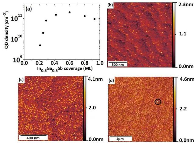
FIG. 3. From left: (a) QD density vs.  $\text{In}_{0.5}\text{Ga}_{0.5}\text{Sb}$  coverage. (b)–(d) AFM micrographs of  $\text{In}_{0.5}\text{Ga}_{0.5}\text{Sb}/5$  ML GaAs on GaP QDs, using 1 s Sb-flush, with increasing QD material supply: 0.21, 0.42, and 1 ML, respectively. In (d) a cluster is marked by a black circle.
