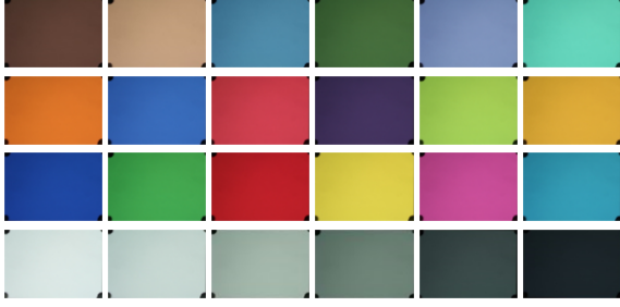
Figure 6: The 24 photographs of the colored patches used for the colorimetric characterization, obtained by projecting the XYZ tristimulus values of a standard color checker on the reflective target.
