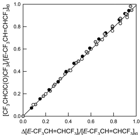
Fig. 7 Formation of  $\text{CF}_3\text{CHClC}(\text{O})\text{CF}_3$  versus the loss of  $E\text{-CF}_3\text{CH}=\text{CHCF}_3$  in the presence of Cl atoms. The shades indicate the  $\text{O}_2$  partial pressure: 16 Torr (white), 140 Torr (gray), and 700 Torr (black) in a total of 700 Torr made up with air or  $\text{N}_2$ .
