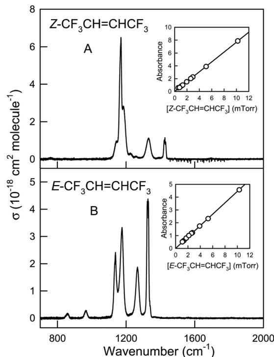
Fig. 12 IR spectra of 1.30 mTorr *Z*- $\text{CF}_3\text{CH}=\text{CHCF}_3$  (panel A) and 2.25 mTorr *E*- $\text{CF}_3\text{CH}=\text{CHCF}_3$  (panel B). The insets show the linearity of the absorbance.
