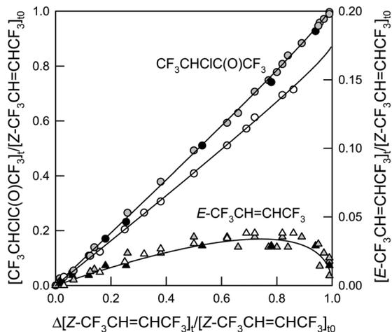
Fig. 9 Formation of  $\text{CF}_3\text{CHClC(O)CF}_3$  (circles, left y-axis) and  $E\text{-CF}_3\text{CH}=\text{CHCF}_3$  (triangles, right y-axis) versus the loss of  $Z\text{-CF}_3\text{CH}=\text{CHCF}_3$  in the presence of Cl atoms in a total of 700 Torr air in the absence (gray) and presence (white) of NO or 700 Torr  $\text{O}_2$  in the absence of NO (black). The lines are non-linear fits to the data. See text for details.
