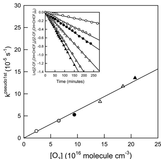
Fig. 4 Pseudo first-order rate coefficients of the reaction  $O_3 + Z-CF_3CH=CHCF_3$  versus  $O_3$  concentration. The inset shows the loss of  $Z-CF_3CH=CHCF_3$  versus time at different  $O_3$  concentrations. The symbols indicate different  $O_3$  partial pressures: 0.73 Torr (white circles), 2.01 Torr (gray circles), 2.91 Torr (black circles), 4.39 Torr (white triangles), 5.71 Torr (gray triangles), and 6.41 Torr (black triangles). See text for details.
