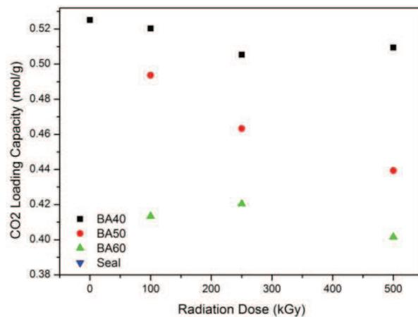
Figure 2. The CO<sub>2</sub> Loading Capacity Against Radiation Dose for All Four Samples
