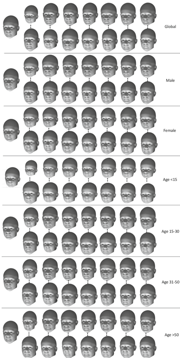
Fig. 20 Global shape model and shape sub-models for age and gender demographics: 1st block—global model; 2nd–3rd block—gender-specific models (male and female); 4th–7th block—four age-specific models (< 15, 15–30, 31–50, > 50). In each block, the mean and the seven most significant shape components are shown: + 3SDs (top row of each block) and – 3SDs (bottom row of each block)
