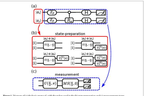
Figure 1. Diagram of (a) the basic protocol, with the pulses used in the (b) state preparation and (c) measurement stages.
