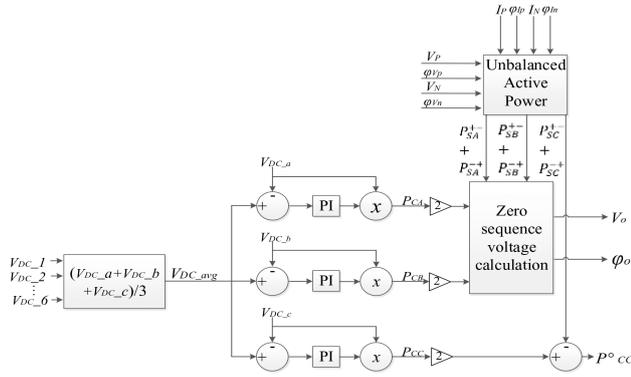
Fig. 6 Cluster Balancing control block diagram
