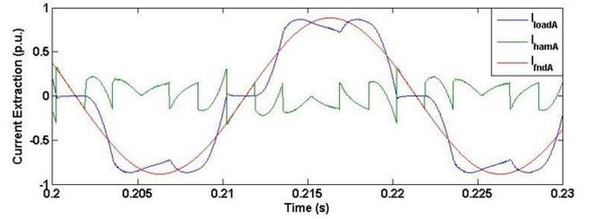
**Fig. 3** Current harmonics extraction from phase-A load current
