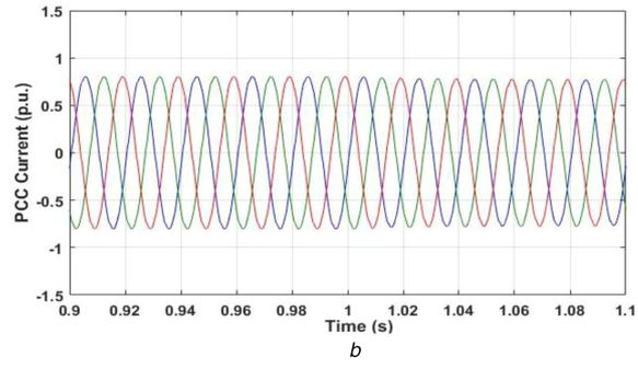
Fig. 8 3-phase PCC current waveform (a) 3-phase PCC current without MMCC-APC compensation and (b) with MMCC-APC compensation
