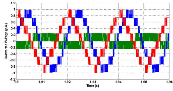
Fig. 9 3-phase converter terminal voltage
