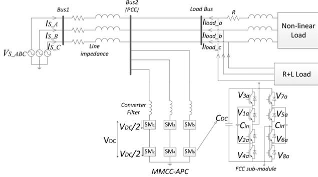
**Fig. 1** MMCC APC circuit and power system diagram
