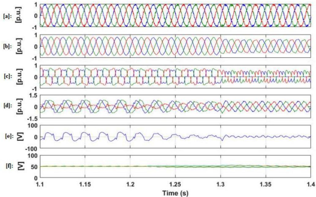
**Fig. 11** Operating results of the MMCC-APC compensation
