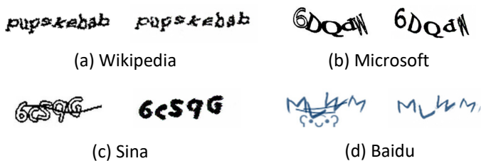
Figure 12: Character segmentation produced by our pre-processing model. For each scheme, the left image is the input captcha, and the right image is the output of our pre-processing model.
