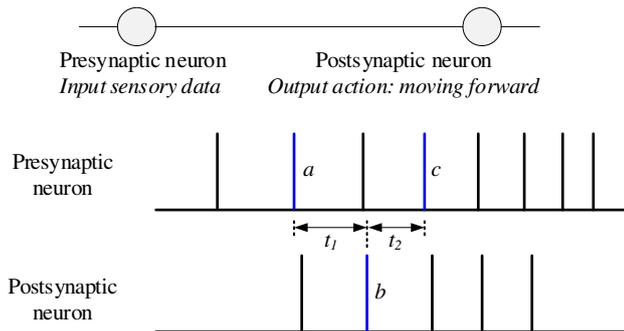
**Fig. 1.** Temporal changing between the input sensory spikes and output spikes for obstacle avoidance where the output neuron is to move forward.
