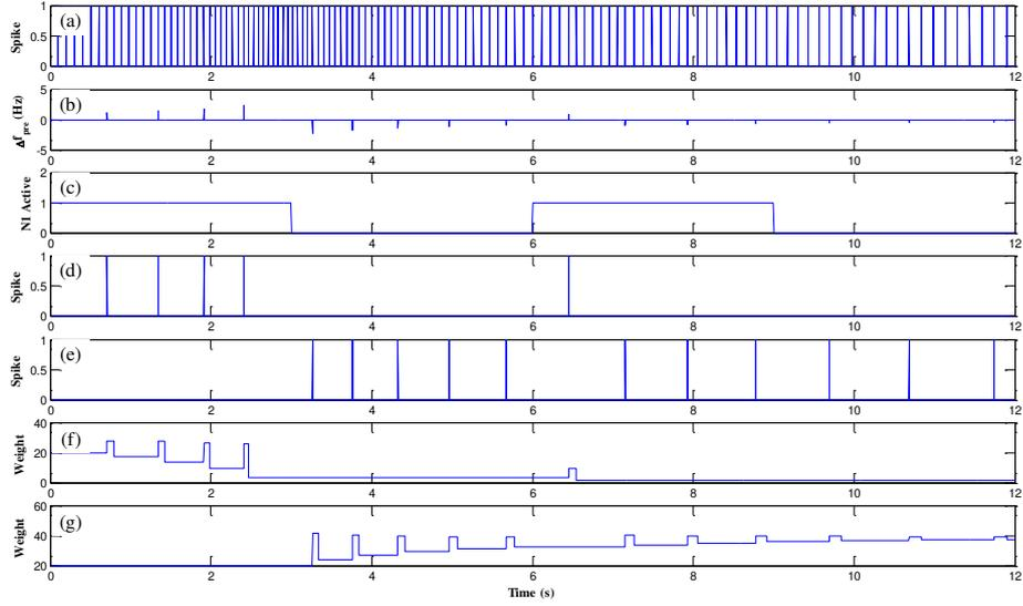
**Fig. 3.** SNN activities between input sensor neuron and output action neurons. (a). Input spike train. (b).  $\Delta f_{pre}$ . (c). Neuron A active status where 1 represents active and value 0 represents inactive. (d, e). Spikes of output neuron A and B. (f, g). Synapse #1 and #2 weights.
