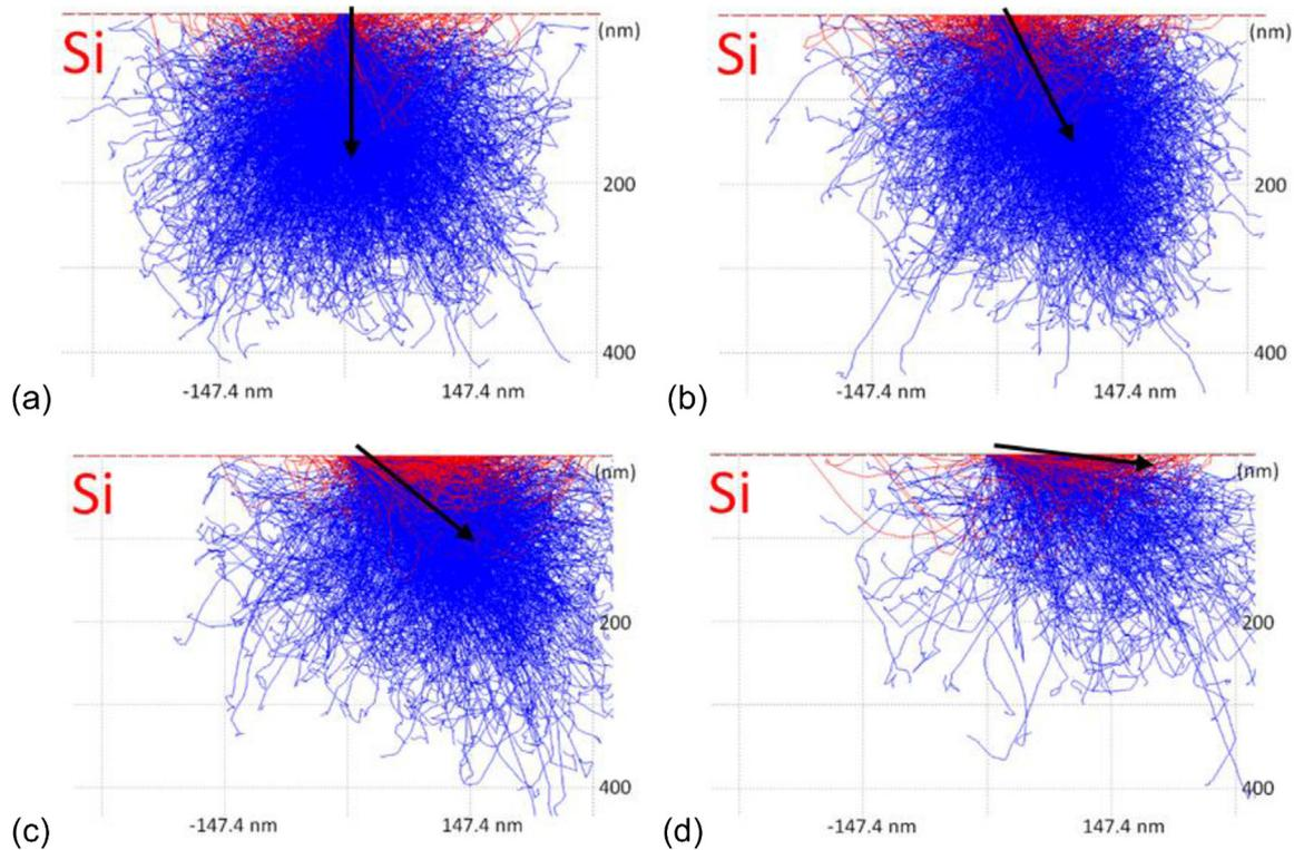
**Figure 4.** Demonstration of the effect of changing angle of incidence,  $\theta$ , on the maximum penetration depth of BSEs and spent electrons, simulated in CASINO. For each case  $\theta$  is (a) 0, (b) 30, (c) 60 and (d) 89°. These incidence angles are indicated by the arrows on the diagram.
