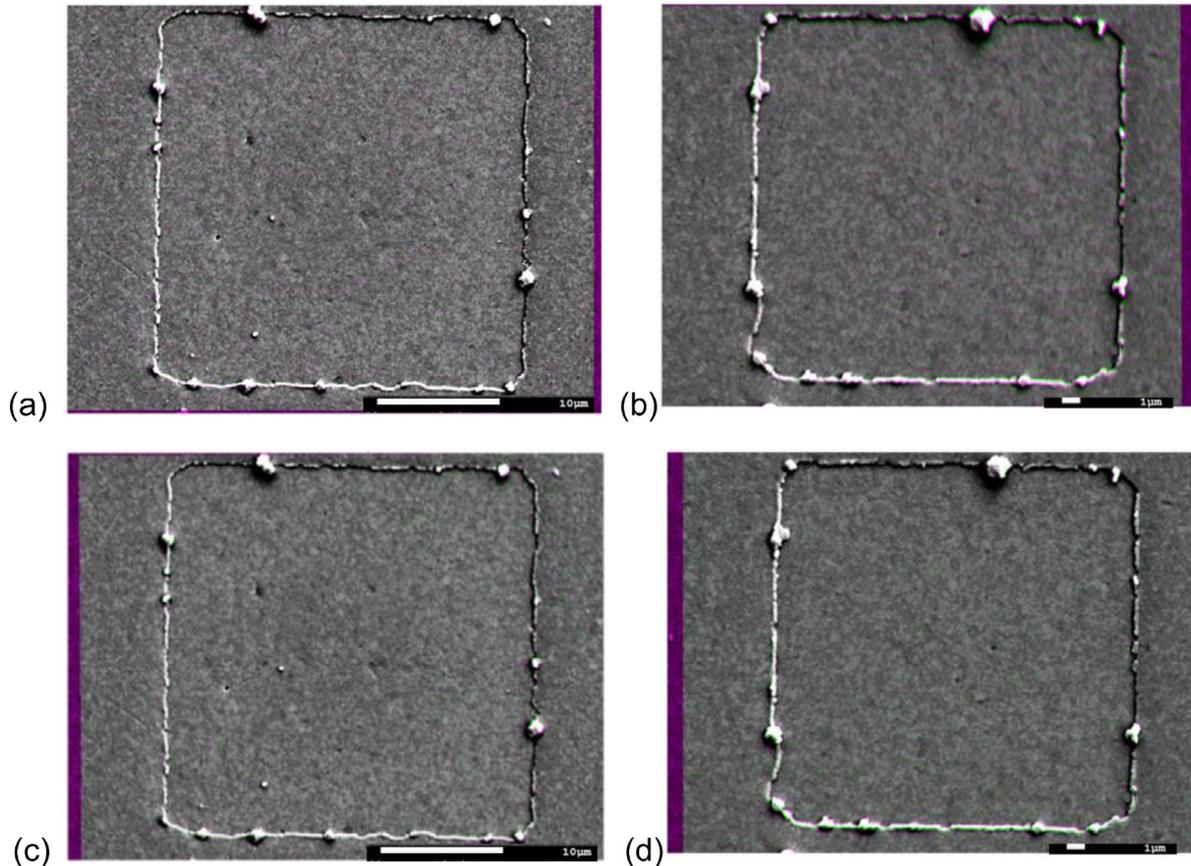
**Figure 6.** Subtracted SEM images focused on the bottom CoFeB/MgO interfaces for (a) high and (b) low TMR MTJs. The corresponding SEM images on the top MgO/interfaces for (c) high and (d) low TMR MTJs.
