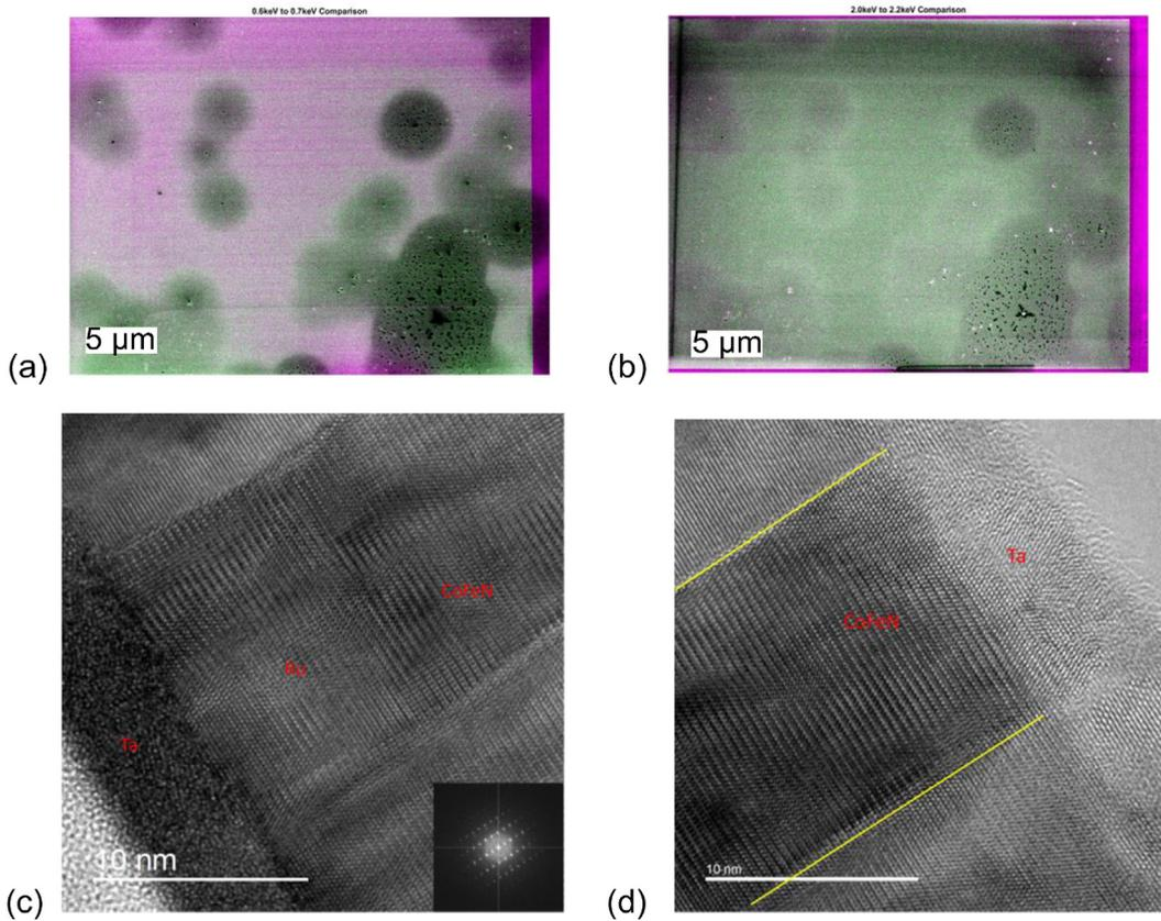
**Figure 7.** SEM images of a Si/SiO<sub>2</sub>//Ta/Ru/CoFe:N/Ta multilayer subtracted between the electron-beam acceleration of (a) 0.6 and 0.7 keV to highlight the CoFe:N/Ta interface and (b) 2.0 and 2.2 keV to highlight the Ru/CoFe:N interface. (c) and (d) Cross-sectional TEM image of the interfaces with the same multilayered structure including a selected area electron diffraction pattern as an inset in (c).
