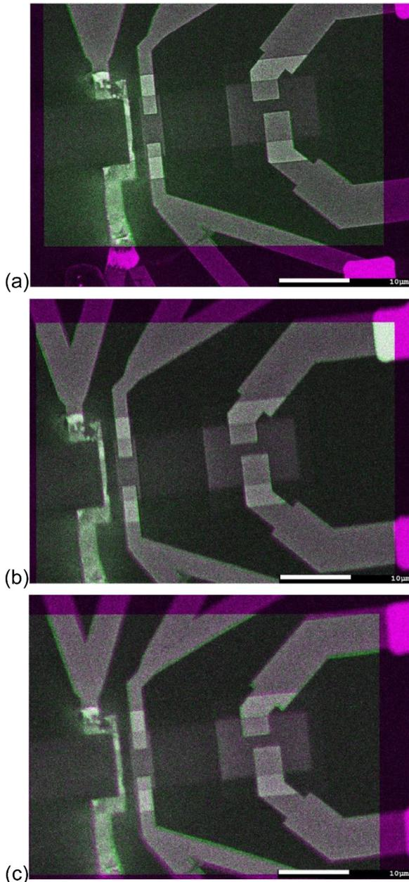
**Figure 9.** *In situ* SEM images of Fe/GaAs lateral spin-valves subtracted between the electron-beam acceleration of 2.5 and 3.0 keV to highlight the interfaces. These images are measured under the current applications of (a) 0.25, (b) 200 and (c) 400  $\mu$ A.
