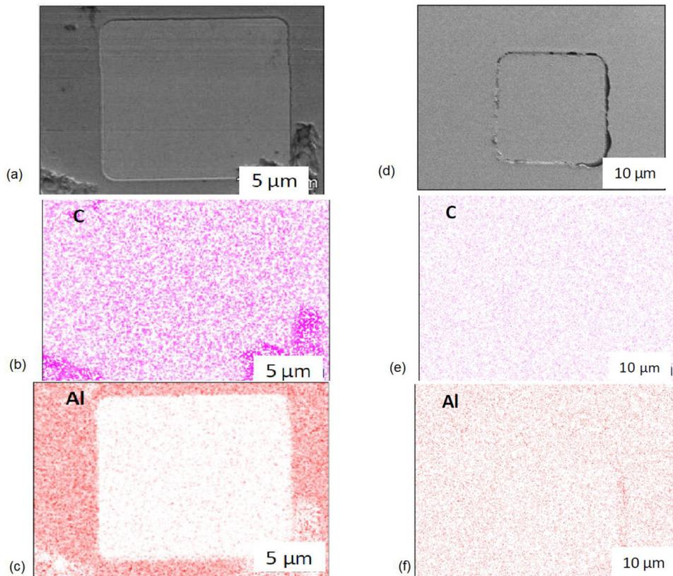
**Figure 5.** (a) and (d) Scanning electron images of a high and low TMR junction, respectively, taken at 10.5 keV. (b) and (c) Elemental maps of the high TMR device. (e) and (f) Elemental maps of the low TMR device. Reproduced from [16]. [CC BY 4.0](https://creativecommons.org/licenses/by/4.0/).
