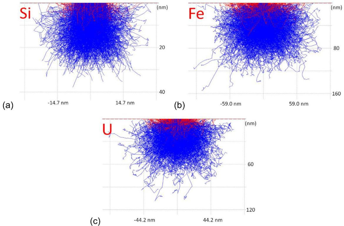
**Figure 3.** Demonstration of the effect of changing atomic number,  $Z$ , on the maximum penetration depth of BSEs and spent electrons, simulated in CASINO. For each case  $Z$  is (a) 14 (silicon), (b) 26 (iron) and (c) 92 (uranium).
