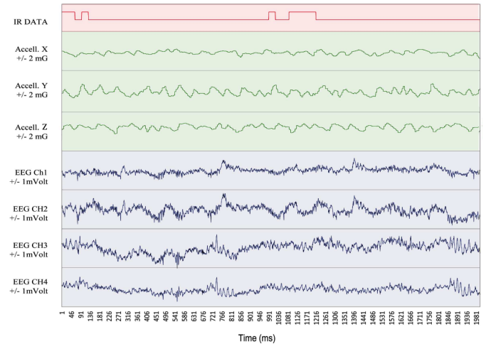
Fig. 9. NAT-1 data capture results, showing infrared data recording (red), accelerometer (green, 3-axis X/Y/Z), and 4-channel EEG programmable field-potential sensing (blue).
