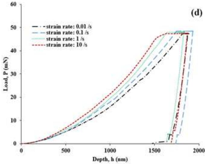
**Figure 4.** Load–displacement curves displaying loading, holding, and unloading portions at different strain rates (0.01–10 /s) for: (a) Pure Mg, (b) Mg–0.25 vol. % CNT, (c) Mg–0.5 vol. % CNT, and (d) Mg–0.75 vol. % CNT.
