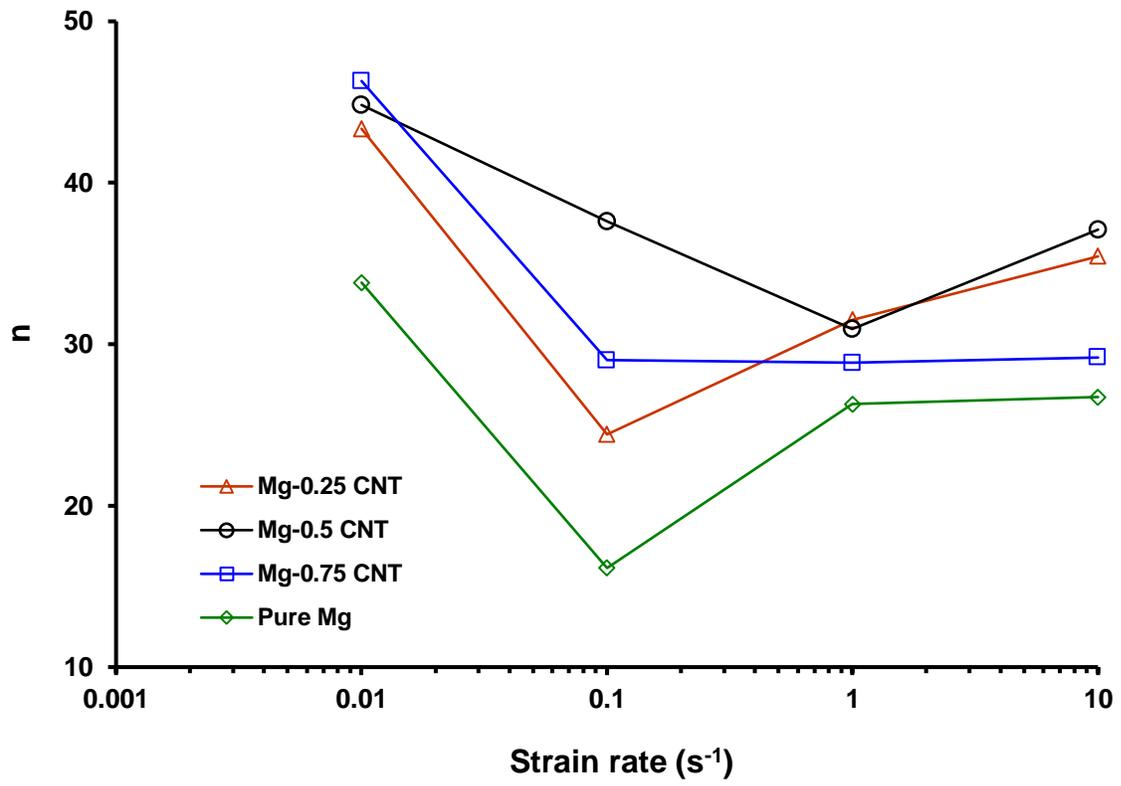
Figure 9. Creep stress exponent (n) values for all strain rates tested.
