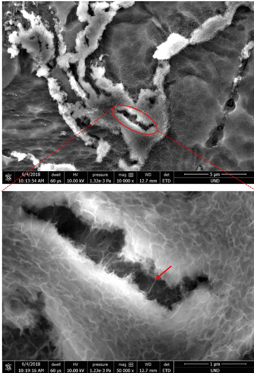
**Figure 2.** Scanning Electron Microscopy (SEM) images of Mg-0.5 v/v % CNT. The higher-magnification image reveals an individual CNT fiber, indicated with an arrow.
