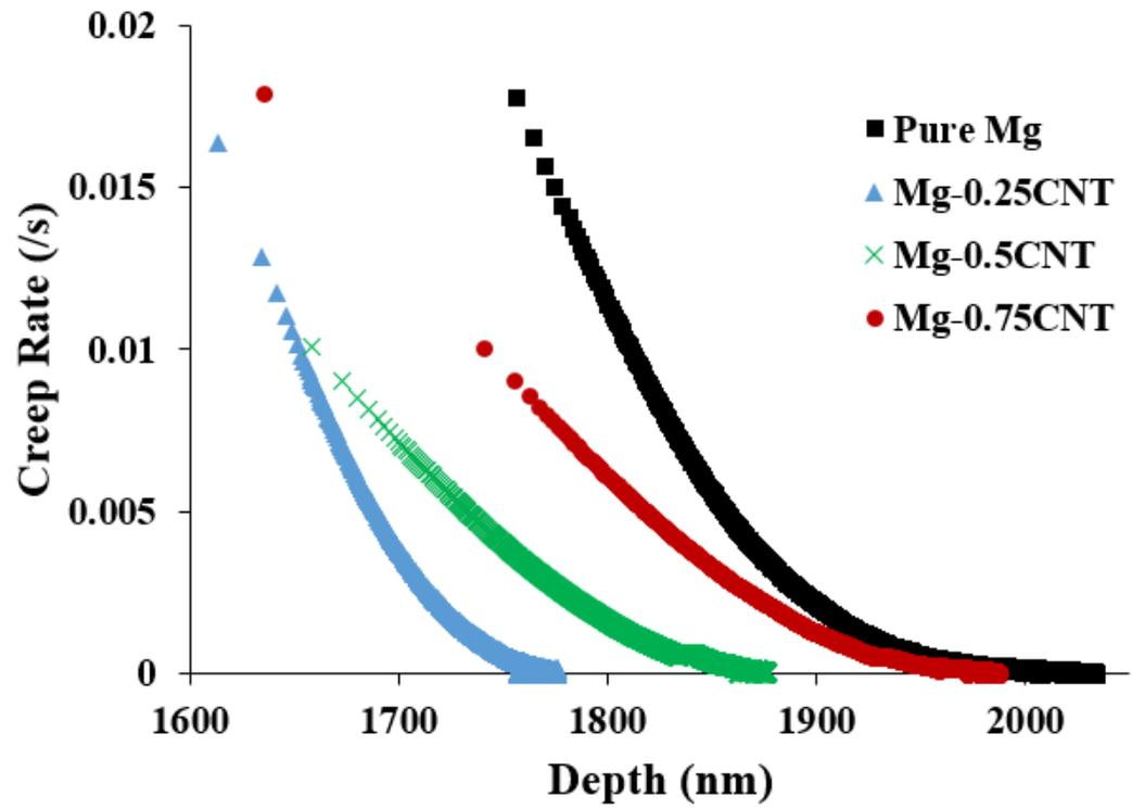
**Figure 10.** Creep rate versus indentation depth for pure magnesium and the Mg-CNT nanocomposites at the strain rate of 10 /s.
