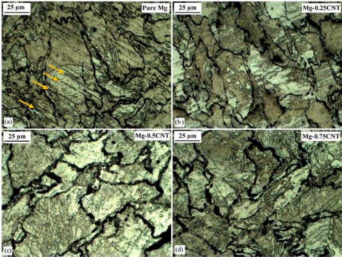
**Figure 1.** Optical micrographs revealing the cross-sectional grain morphologies of (a) Pure Mg, (b) Mg-0.25 v/v % CNT, (c) Mg-0.5 v/v % CNT, and (d) Mg-0.75 v/v % CNT. Arrows are added to (a) to show the mechanical twins present in pure Mg.
