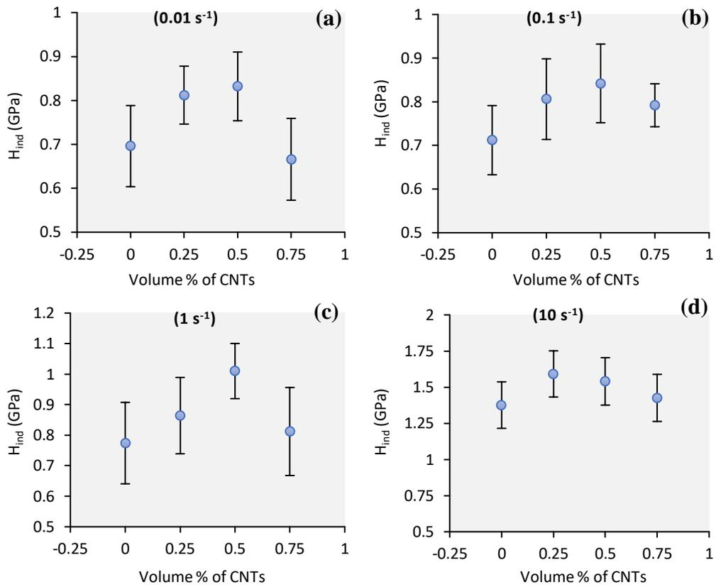
**Figure 6.** Variation of indentation hardness as a function of CNT loading over four strain rates: (a)  $0.01 \text{ s}^{-1}$ , (b)  $0.1 \text{ s}^{-1}$ , (c),  $1 \text{ s}^{-1}$ , and (d)  $10 \text{ s}^{-1}$ .
