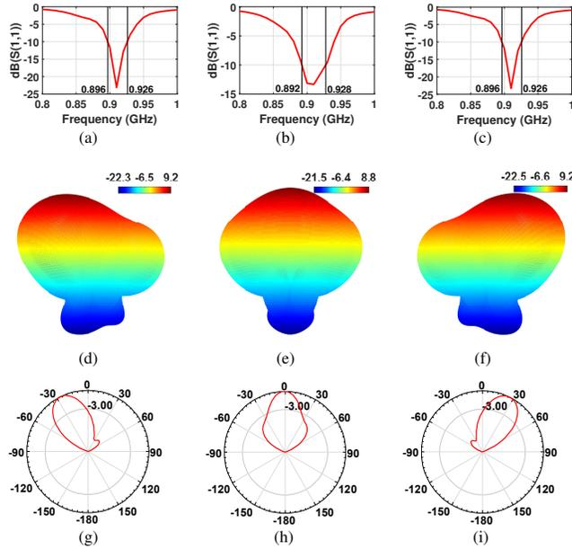
**Figure 4: Frequency and radiation properties of our reconfigurable antenna system. Here (a-c), (d-f) and (g-i) respectively represent the frequency property, radiation pattern and normalized radiation pattern of mode1-3.**
