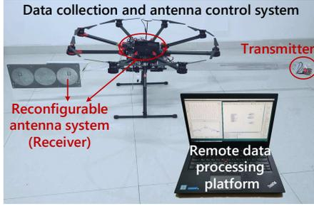
**Figure 2: Overview of WIDEEE.** We use a drone to carry the LoRa transceiver pair and its control system. The data are sent back to the remote data processing platform to perform real-time target detection and localization.
