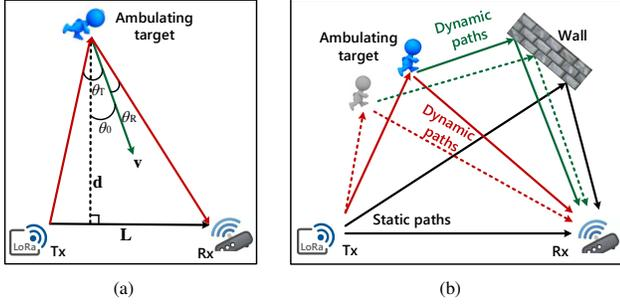
**Figure 8: (a) shows the setup of moving target localization. Similar to the linear virtual array constructed by moving receiver. The moving target also can emulate a linear array. (b) presents the superposition signal of multiple paths.**
