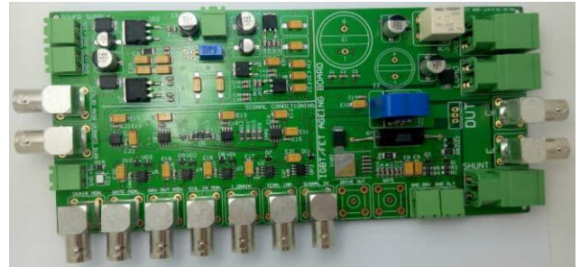
Fig. 3. Accelerated Ageing System Custom Built PCB
