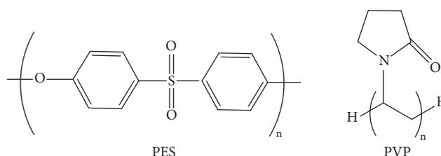
FIGURE 2: Chemical structure of PES and PVP.
