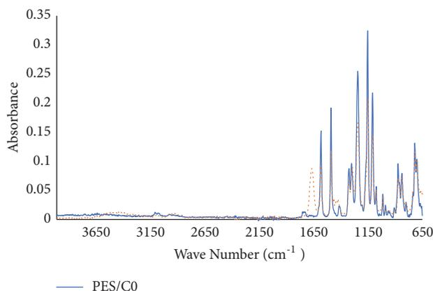
FIGURE 8: Fourier transform infrared spectrum of PES/C.
