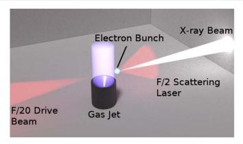
**Figure 1.** A schematic of an all-optical inverse Compton scattering setup. An F/20 drive laser (intensity  $\sim 10^{19}$  W cm<sup>-2</sup>) is focused into a supersonic gas jet, producing an electron bunch via wakefield acceleration. These electrons then collide with a counter-propagating F/2 laser pulse (of high intensity  $\sim 10^{21}$  W cm<sup>-2</sup>). The scattered electrons produce a bright x-ray beam.
