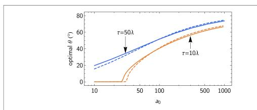
**Figure 2.** The angle at which  $\chi_{\text{max}}$  is largest, as predicted by (4): for a collision between an electron beam with  $\gamma_0 = 2 \times 10^4$  (solid) and  $5 \times 10^3$  (dashed) and a laser pulse with given  $a_0$ , wavelength  $\lambda = 0.8 \ \mu\text{m}$ , spot size  $r_0 = 2 \ \mu\text{m}$  and duration  $\tau = 50\lambda$  (blue) and  $10\lambda$  (orange).
