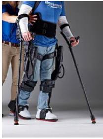
Fig. 5. EksoGT exoskeleton with a patient inside [17].
