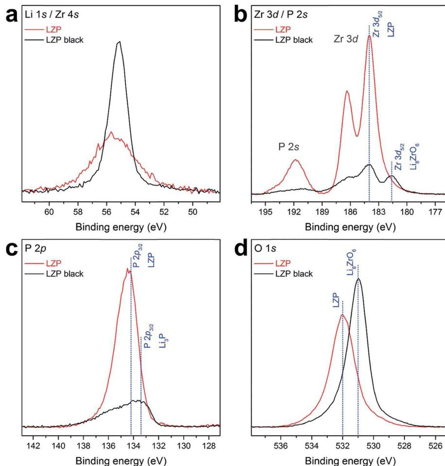
Fig. 7 XPS core levels of LZP-1100 and the black surface layer (LZP black) formed after cycling a Li/LZP/Li cell at  $80^\circ\text{C}$  for 100 h, including (a) Li 1s/Zr 4s, (b) Zr 3d/P 2s, (c) P 2p, and (d) O 1s.
