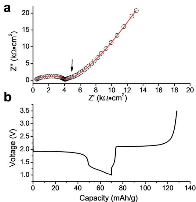
Fig. 9 (a) The impedance spectrum collected from the Li/LZP/LTP cell (LTP pellet thickness  $\sim 0.9$  mm) at 50 °C; the arrow indicates an intermediate-frequency semicircle assigned to the LTP/LZP interfacial resistance. (b) Discharge/charge profile of the Li/LZP/LTP cell at 50 °C and  $6 \mu\text{A cm}^{-2}$ .
