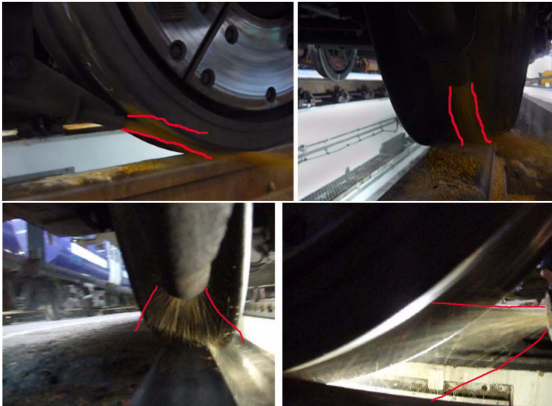
Figure 18 – (Top) Narrow Discharge Pattern vs (Bottom) Wide Discharge Pattern. 5
