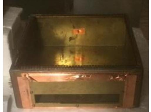
Fig.3. Photo of the Enclosure used in the Measurements with its Lid Removed.
