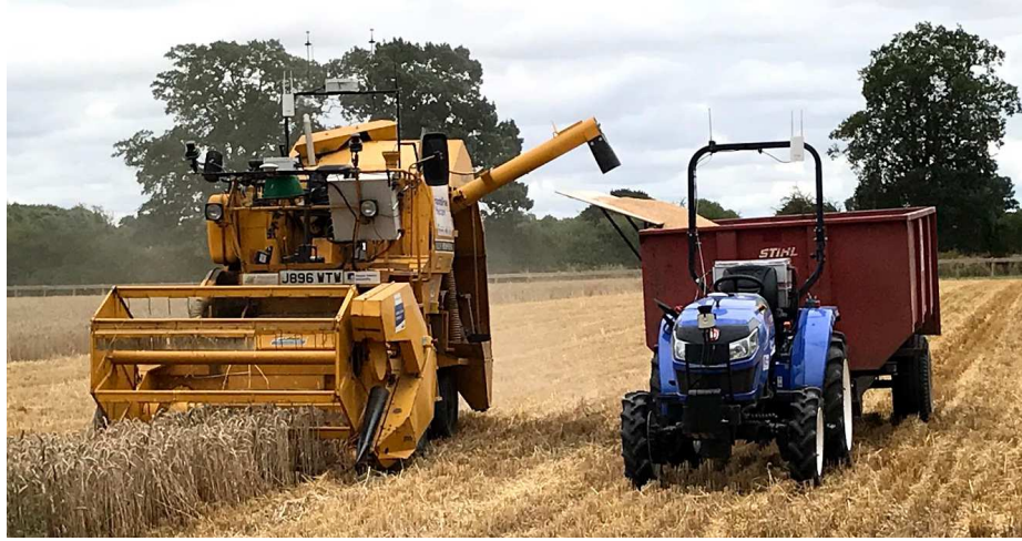
Fig. 1. Hands Free Hectare autonomous harvest using a Sampo Rosenlew 130 combine harvester and an Iseki compact tractor retrofitted with GPS autopilot hardware.
