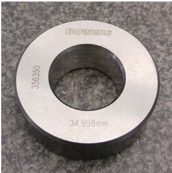
(c) Micrometre metric setting ring
