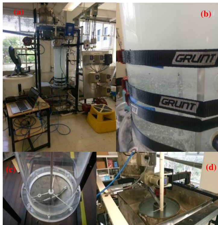
Figure 2 a) Overall view of the setup used for the laboratory-scale thickener experiments, b) the observed flocs during operation, c) the rake and funnel section, and d) the feedwell.
