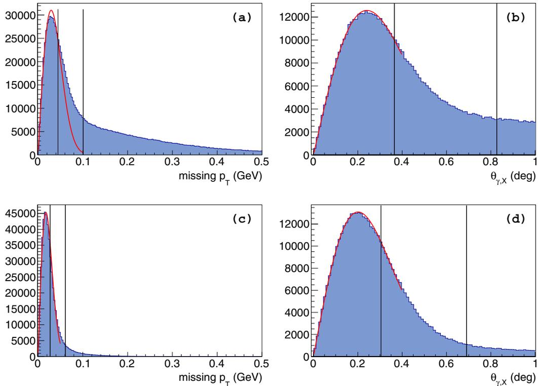
FIG. 10. The same as for Fig. 9 but for  $N(p_T)$ , upper left (a), and  $N(\theta_{\gamma,x})$ , upper right (b). The lower graphs, (c) and (d), respectively, are the same distributions for Monte Carlo-generated data. The distributions for  $N(p_T)$  and  $N(\theta_{\gamma,x})$  were fit with empirical functions of the form  $A \sin(x\sigma) e^{(55 \tan(x\mu)/\sigma)^2}$ .
