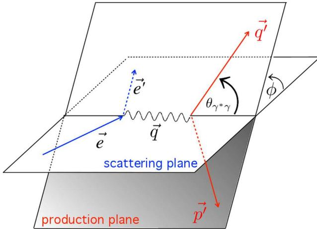
FIG. 2. The electron scattering plane and the plane of the produced photon  $\vec{q}'$ , and recoil proton,  $\vec{p}'$ , respectively, in DVCS. The angle between the photon plane and electron plane is  $\phi$ .
