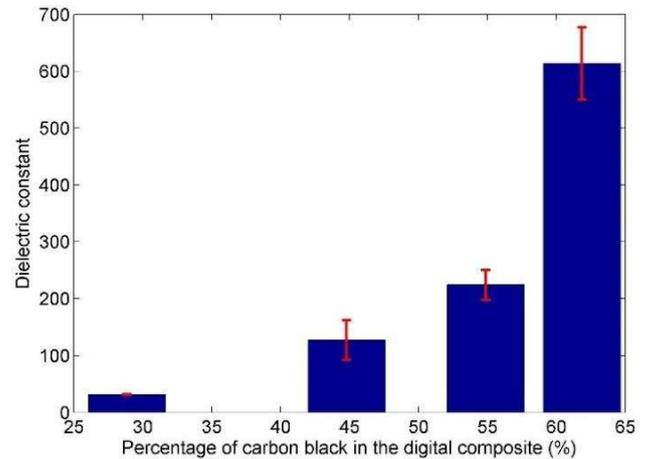
Figure 3, Dielectric constant change against carbon content at a frequency of 1 kHz.
