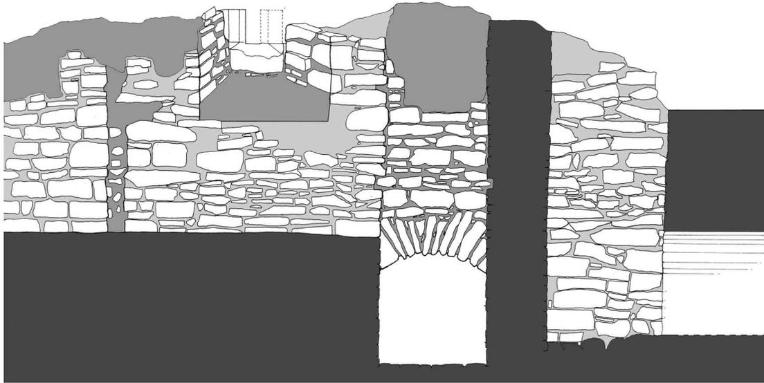
**FIGURE 6-2** West section building elevation of wall (5036), showing the lancet window and garderobe (5051).
