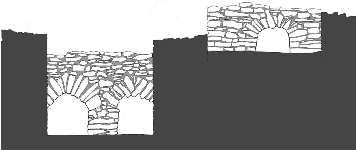
**FIGURE 6-3** North section building elevation showing the double-arched opening (5054) of garderobe (5056) (left) and opening (5052) of garderobe (5041) (right).
