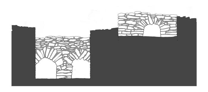
FIGURE 6-3 North section building elevation showing the double-arched opening (5054) of garderobe (5056) (left) and opening (5052) of garderobe (5041) (right).
