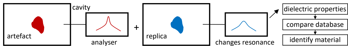
Figure 1. Principle of Dielectric Replica Measurement (DRM)
