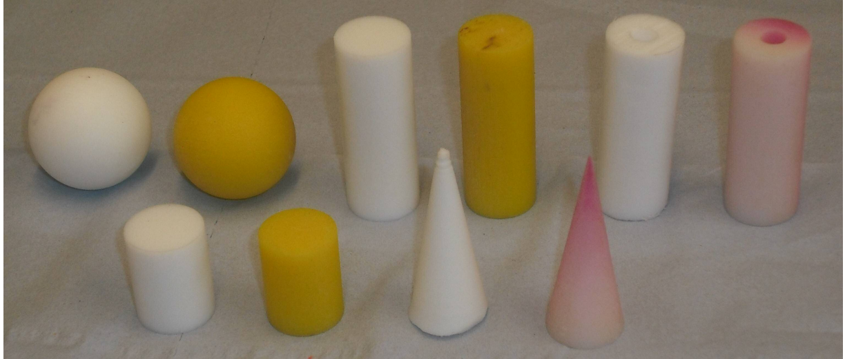
Figure 2. Objects used to test Dielectric Replica Measurement (DRM), with PTFE versions to left of 3D-printed acrylic copies. The sphere at the top left is 25.6mm in diameter.
