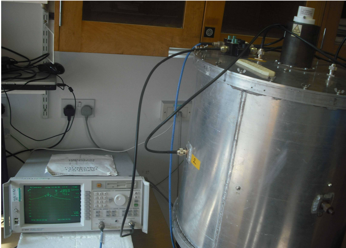
Figure 3. Photograph of cavity (right) connected to VNA (left). One of the connectors probing the horizontal, TE 111 mode, for x- and y-perturbations, can be seen on the left side of the cavity. The end of the rotatable sample holder (white) is at top right.
