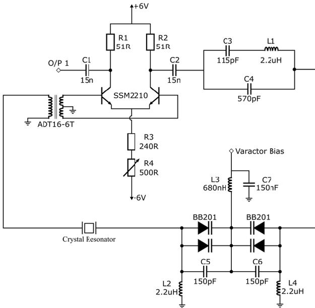
Fig. 17. 10-MHz crystal oscillator complete circuit diagram.
