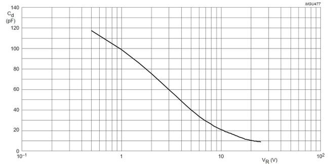
Fig. 13.  $C-V$  characteristics for BB201.
