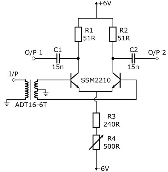
Fig. 4. Differential amplifier circuit diagram.
