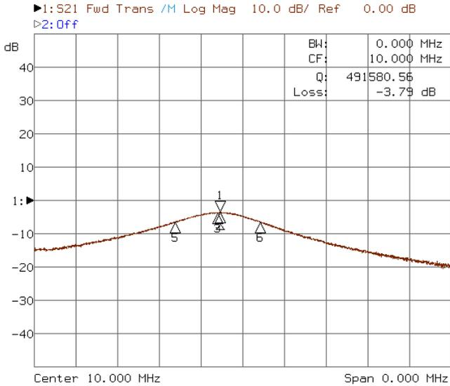
Fig. 7. Crystal resonator series resonance (span = 100 Hz).
