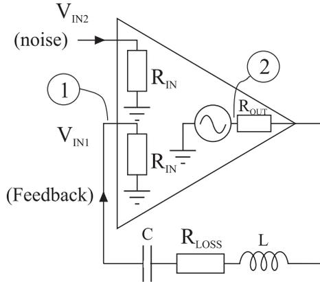
Fig. 1. Oscillator model.
