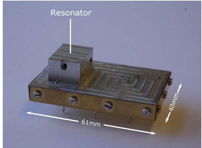
Fig. 18. Crystal oscillator in aluminum jig (Oscillator 2).
