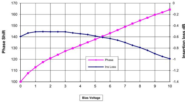
Fig. 15. Insertion loss and phase shift versus voltage.
