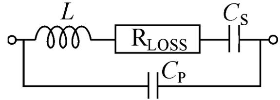
Fig. 6. Model for crystal resonator.
