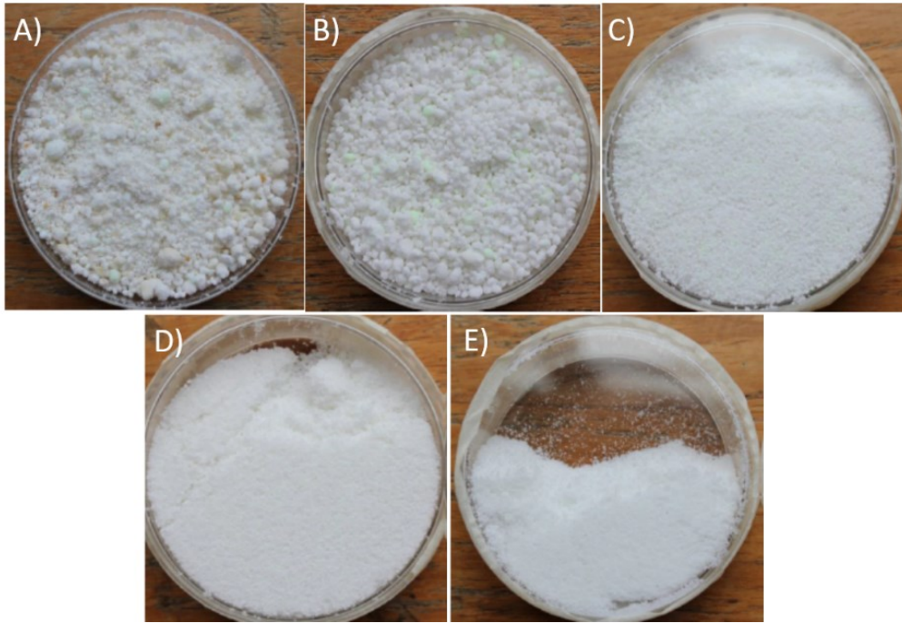
Figure 4. Digital images of a detergent powder sample as a function of particle size; a) unsieved sample, b) above 841 microns, c) 500 - 841 microns, d) 250 - 500 microns and e) below 250 microns. These correspond to samples 10 to 14 in the supplementary information.
