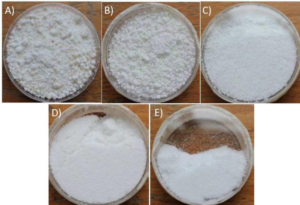
Figure 4. Digital images of a detergent powder sample as a function of particle size; a) unsieved sample, b) above 841 microns, c) 500 - 841 microns, d) 250 - 500 microns and e) below 250 microns. These correspond to samples 10 to 14 in the supplementary information.
