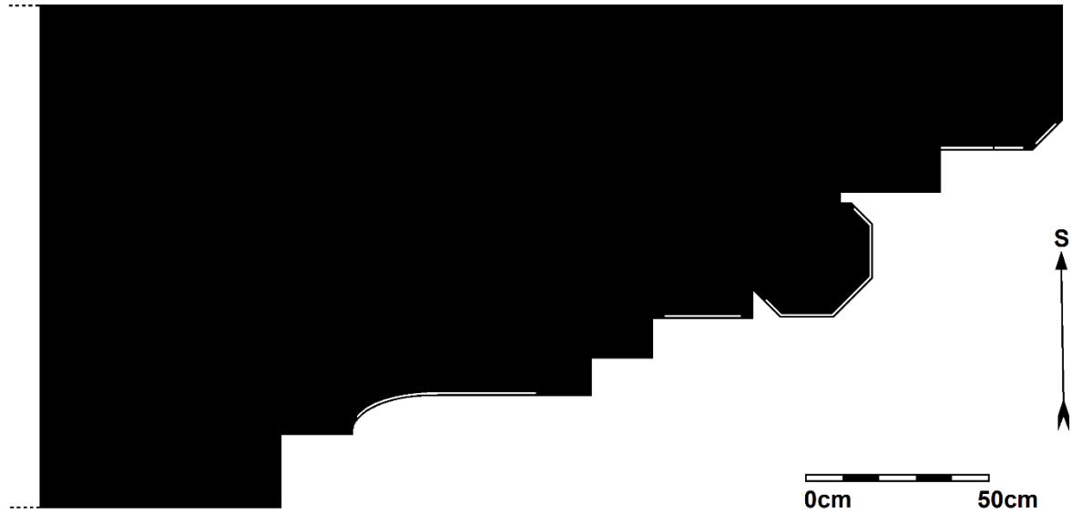
Fig. 4 – Citadel Mosque, Divriği; portal cross-section @ 130cm above top step © R.McClary
