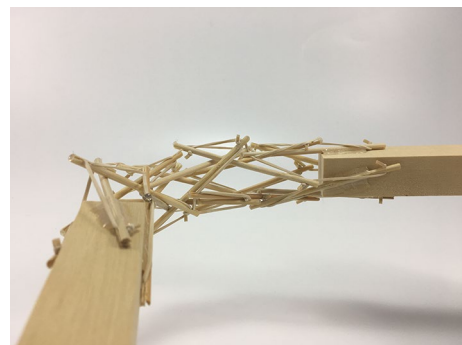
Fig. 47 Hard transitional region prototype. Spiral tensegrity mast
