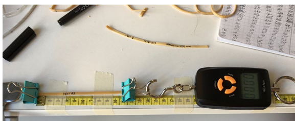
Fig. 56 Rubber band test setup
