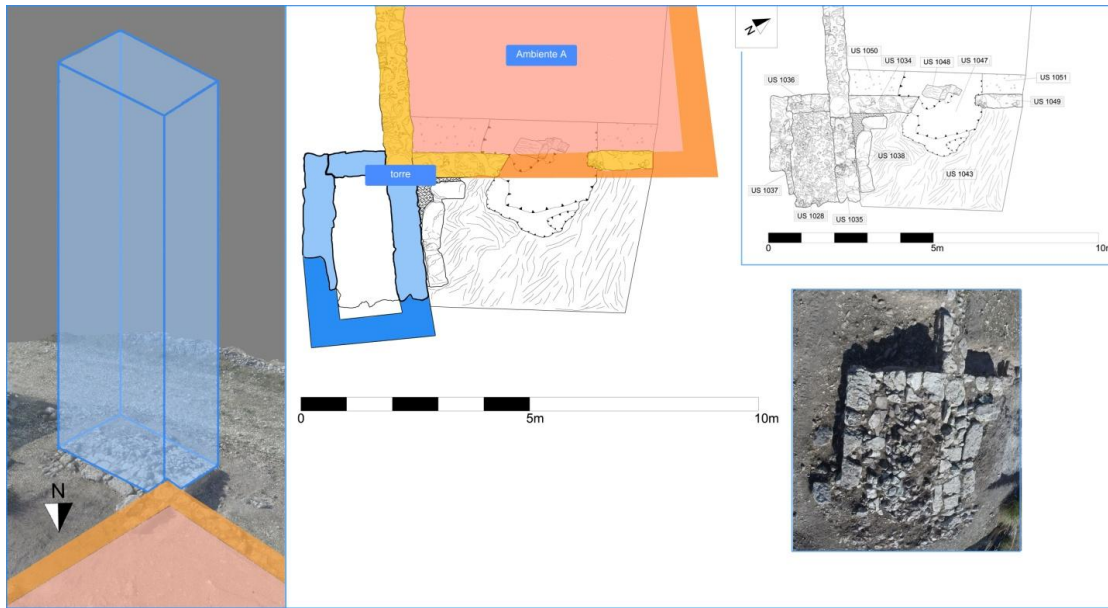
Fig. 5. Surviving elements and reconstruction of the tower standing at the corner of Building B.
