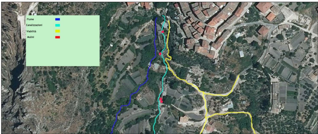
Fig. 9. Model of the hydraulic system in the valley below Fonte Rabato. In blue: river; in yellow, lines of natural drainage; in green the artificial water channel; In red: mill sites.
