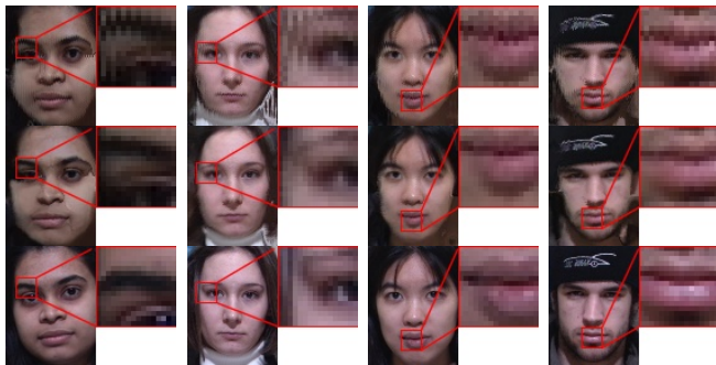
Fig. 12. Comparison of face synthesis results with l_2 (first row) and l_1 (second row) loss terms. While the last row represents the ground truth.
