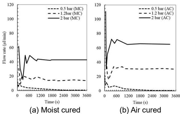
**Figure 5.** Air flow rates under different test pressure
