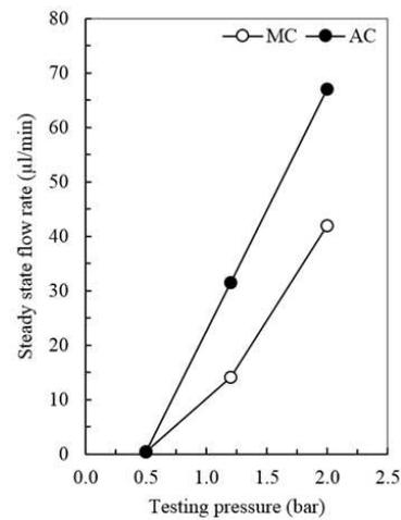
**Figure 6.** Relationship between test pressure and steady state air flow rate (The air flow rates at different pressure were converted to the flow rates at 1 atm)
