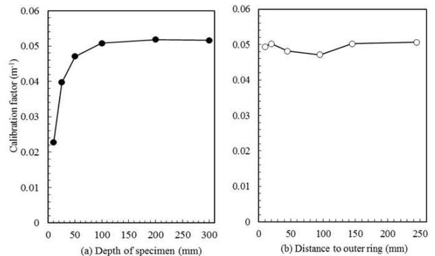
**Figure 3.** Calibration factor under different specimen depths and distances to outer side of the seal
