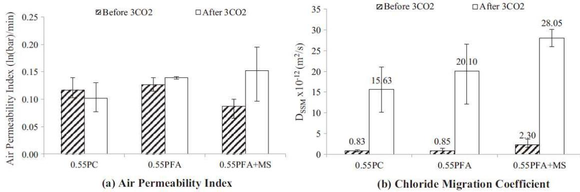
**Figure 8 Influence of carbonation on air permeability and chloride migration coefficient of different types of concrete [Wang et al, 2017]**
