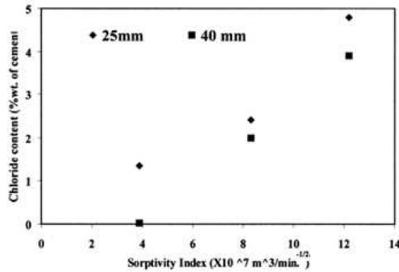
**Figure 4 Relationship between sorptivity index and chloride content at two different depths [Basheer *et al.*, 2008]**
