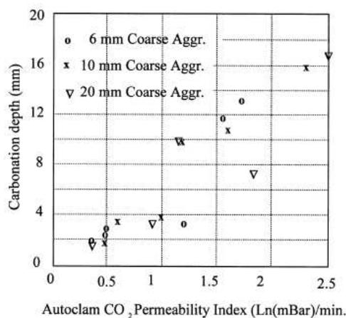
(a) API (Autoclam) VS carbonation depth
