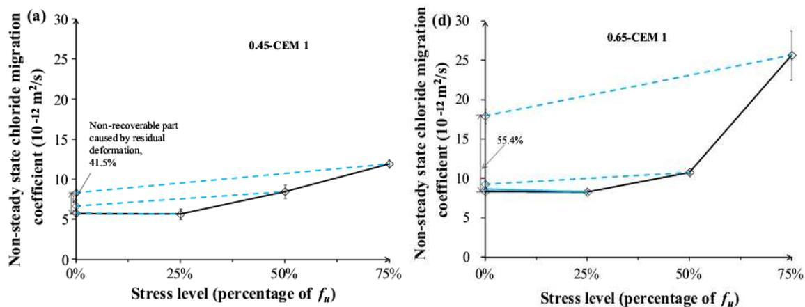
**Figure 6 Relationship between stress level applied and non-steady state chloride migration coefficient [Wang *et al*, 2016]**
