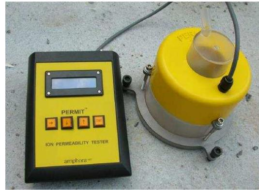
(b) The PERMIT ion migration test apparatus
