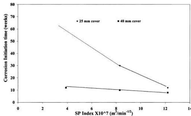
**Figure 5 Relationship between sorptivity index and corrosion initiation time [Basheer *et al.*, 2001]**
