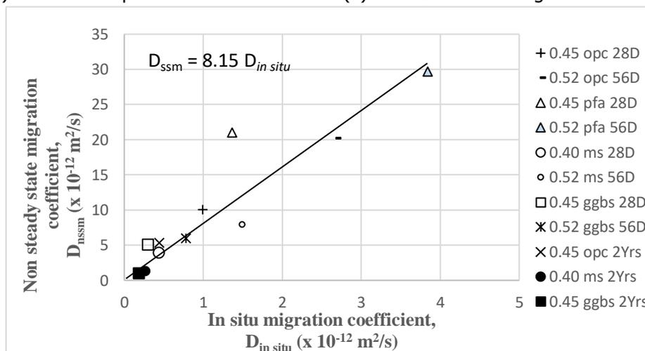
(c) Correlation between Permit in situ migration coefficient and effective diffusion coefficient (all Portland cement mixes; a/c represents aggregate cement ratio)
