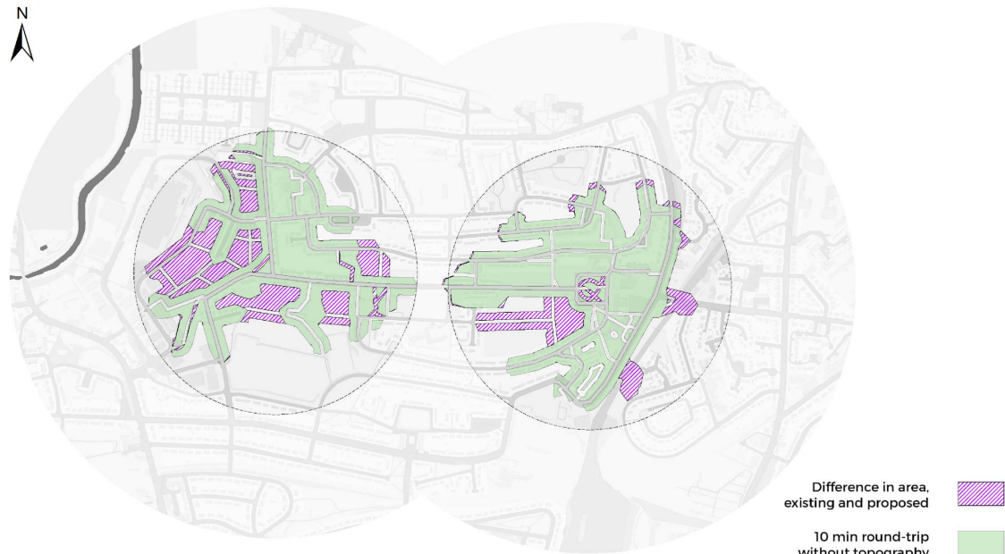
Figure 8. The much denser proposed street network around the western node increases the walkable 10-minute roundtrip catchment by 26%.
