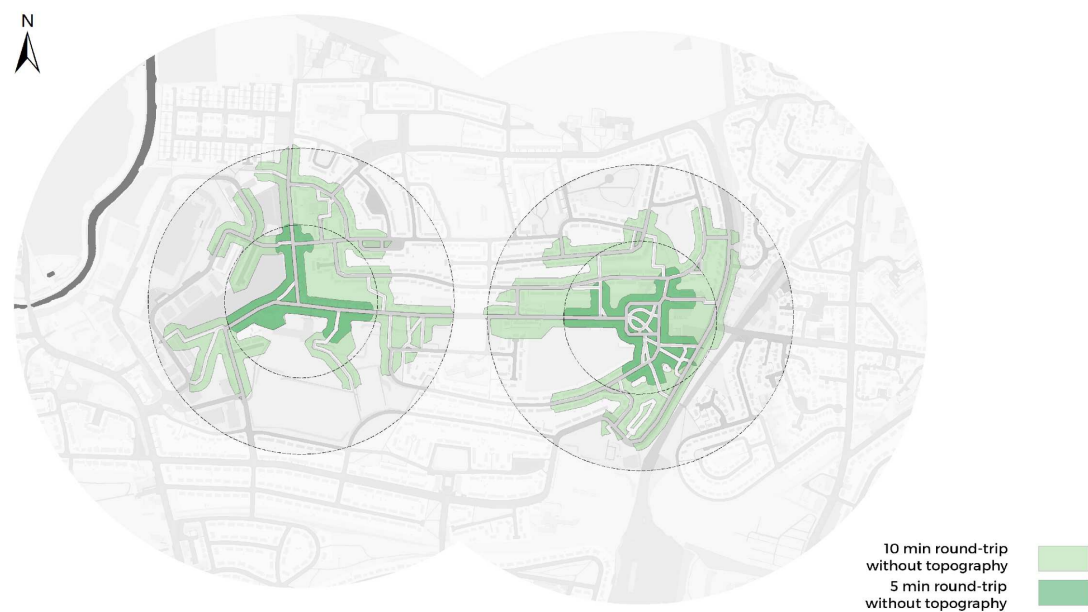
Figure 9. 5- and 10-minute walkable catchments following the existing network, without accounting for topography.
