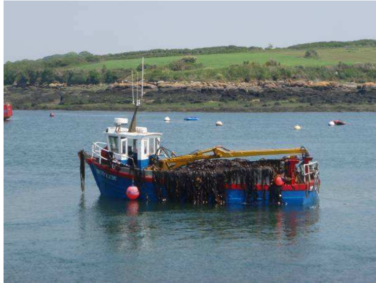
Figure 31. Typical Scoubidou vessel operating in Brittany, France (source: Mesnildrey et al., 2012)
