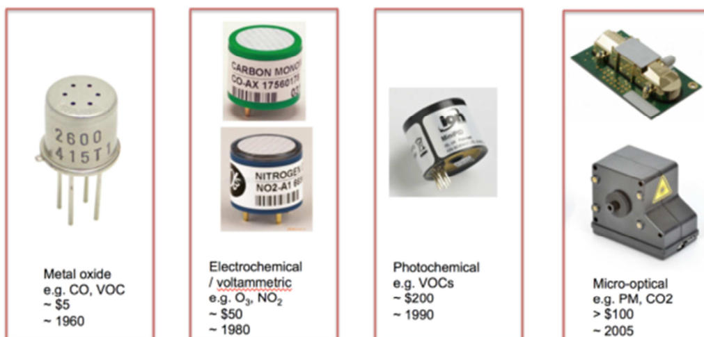
Figure 1. A range of typical low-cost sensor components, example measurement compounds, and approximate cost
