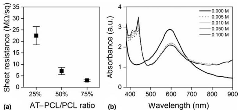
**FIG. 1.** Electrical and optoelectronic characterization of AT-PCL. (a) Sheet resistance of electrospun membranes, produced at different AT-PCL to PCL ratios and doped with 0.1 M HCl. (b) Spectra of AT-PCL in DMSO doped with phytic acid at different molarities.
