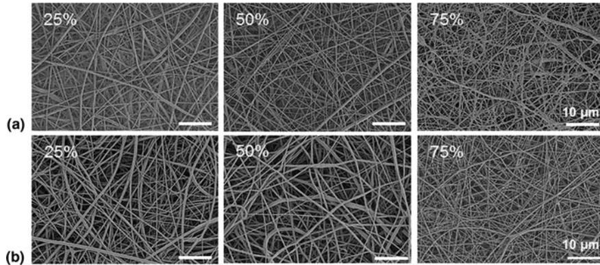
**FIG. 2.** SEM images of fibrous membranes. AT-PCL was blended at different w/w ratios (25%, 50%, and 75%) with high molecular weight PCL and processed by electrospinning. For all AT-PCL to PCL ratios, free standing membranes were produced. (a) Pristine AT-PCL membranes, (b) phytic acid-doped AT-PCL membranes.
