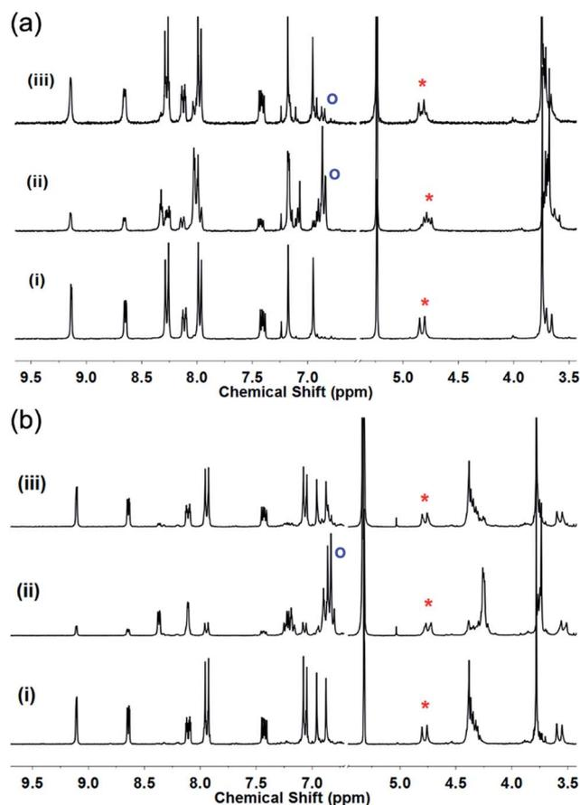
Fig. 2  $^1\text{H}$  NMR spectra (300 MHz) in  $\text{CD}_2\text{Cl}_2$ . (a) Ligand **L2** and (b) ligand **L4** showing in each case (i) initial spectrum, (ii) after irradiation with 355 nm laser to *Z*-rich form; (iii) after irradiation with 450 nm light to return to *E* state. Red asterisk indicates CTG–CH<sub>2</sub>– proton and blue circle indicates aromatic proton shielded in *Z*-isomer.
