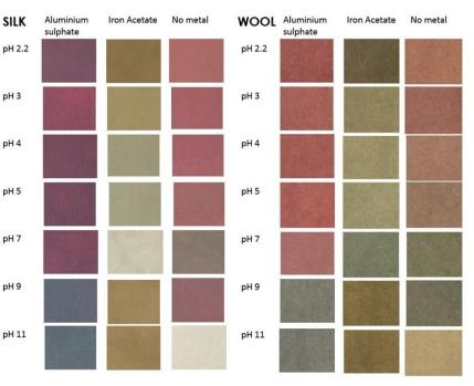
After washing, the majority of silk and wool samples were rated grade 5, indicating no difference between washed and unwashed sample. Light-fastness without metal-complex formation was poor. The best results were obtained when silk and wool were dyed with the addition of  $Fe^{3+}$ , and certain pH combinations with  $Al^{3+}$  and were rated with grade 3.
