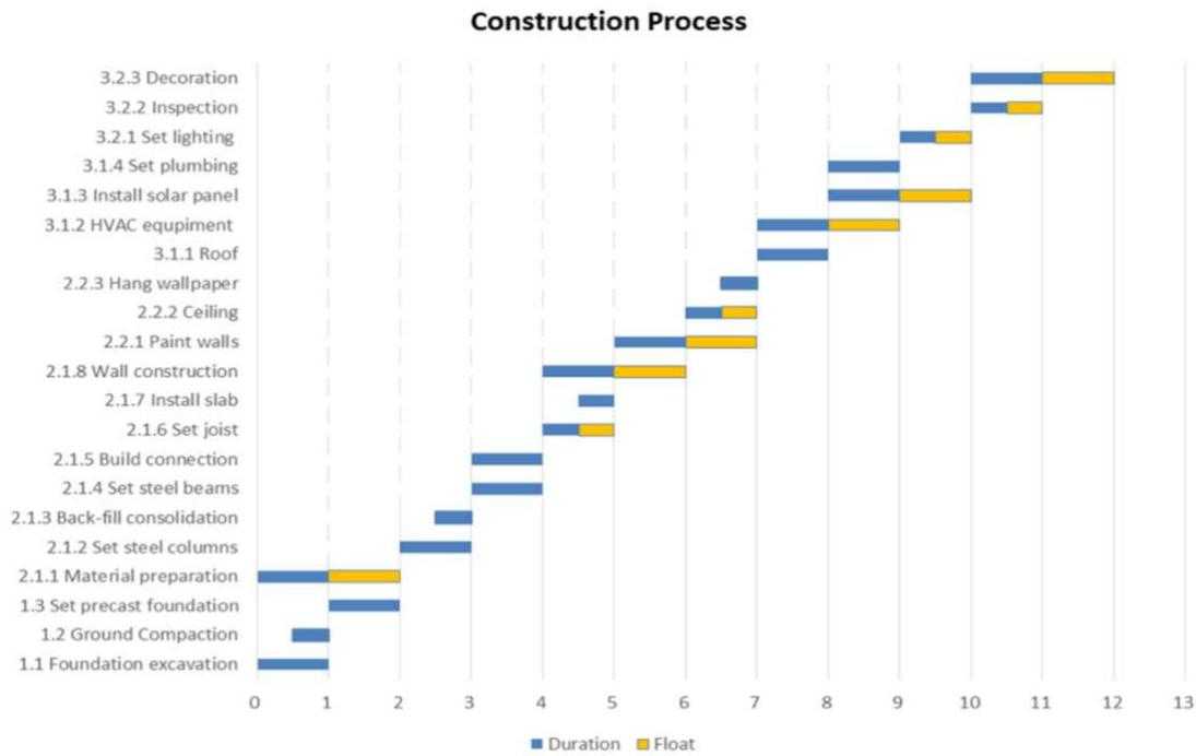
Fig. 13. A demonstration of 12-day on-site construction scheduling
