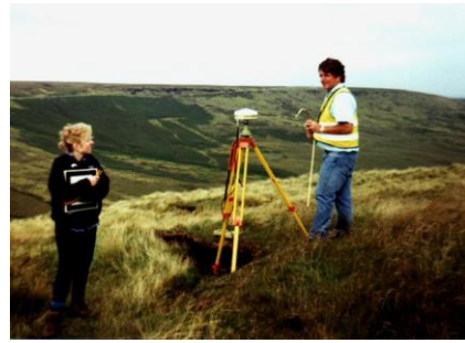
Setting up the survey points using a Satellite Positioning System.
