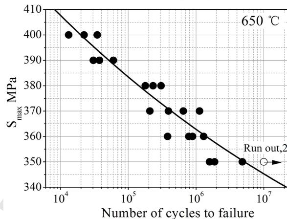
Fig. 13. S-N curves of 23-8N steel at 650 °C.
