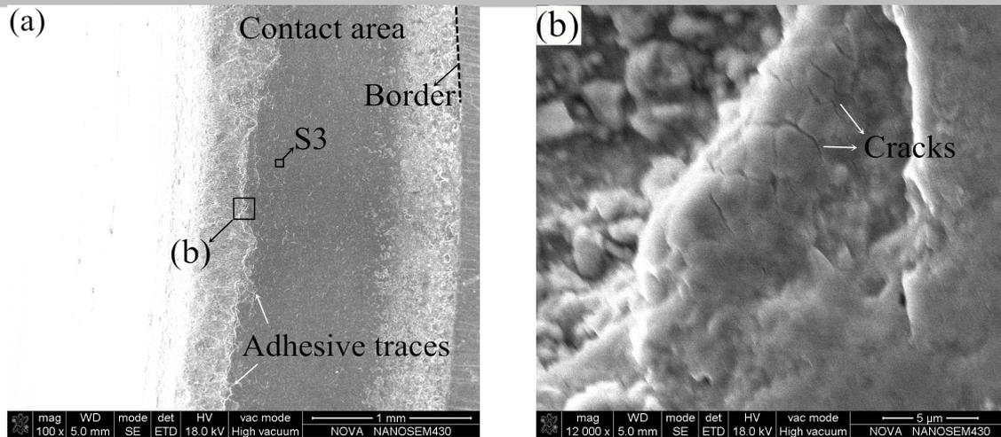
Fig. 25 (a), (b) Worn surfaces of seat insert 3 and EDS test area S3.
