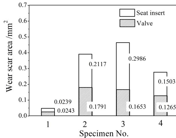
Fig. 19. Total wear of valve and seat insert.
