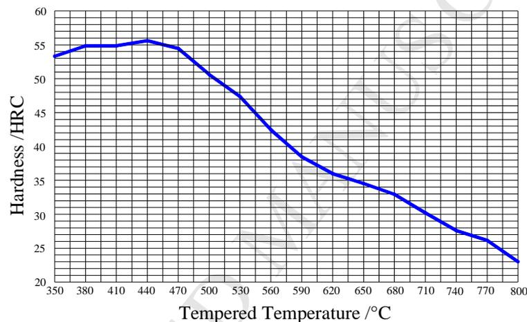
Fig. 10. The calibration curve of quenched 45Cr9Si3 steel.
