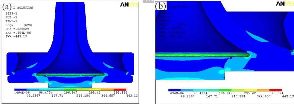
Fig. 12. Stress analysis results by FEM with a load of 4.2 kN.
