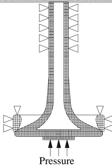
Fig. 8. Schematic diagram of HHSV FEM model.
