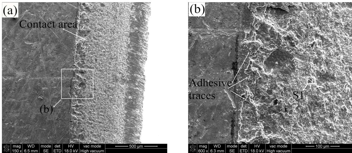
Fig. 23 (a), (b) Worn surfaces of seat insert 1 and EDS test area S1.
