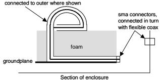
Fig.2 Showing construction method the loops and RC (internal dimensions of
