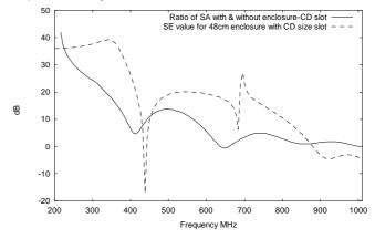
Fig. 14. Comparison of the computed reduction in absorbed power with the SE data for the 480 mm by 480 mm by125 mm enclosure with the CD sized aperture.
