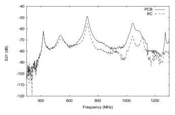
Fig. 4. Comparison of the frequency response of a cavity loaded with a PC controller card (PCB) and an RC of the same size (RC).
