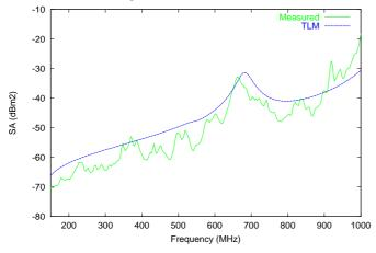
Fig. 10b. Measured and computed SA of a 300 mm by 300 mm by 120 mm enclosure with a floppy disk sized aperture.
