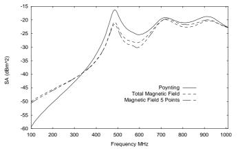
Fig. 5. Comparison of the results of 3 methods of computation of SA
