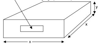
Fig. 9. Showing layout of enclosures with position of aperture (x and y are either 300 mm and 120 mm or 480 mm and 125 mm respectively depending on the enclosure used)
