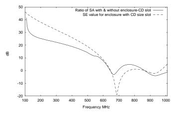
Fig. 11a. Comparison of the computed reduction in absorbed power with the SE data for the 300 mm by 300 mm by120 mm enclosure with the CD sized aperture.
