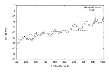
Fig. 8. The effective Shielding Aperture of the Representative Contents with no enclosure present.
