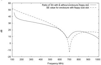
Fig. 11b. Comparison of the computed reduction in absorbed power with the SE data for the 300 mm by 300 mm by120 mm enclosure with the floppy disk sized aperture.
